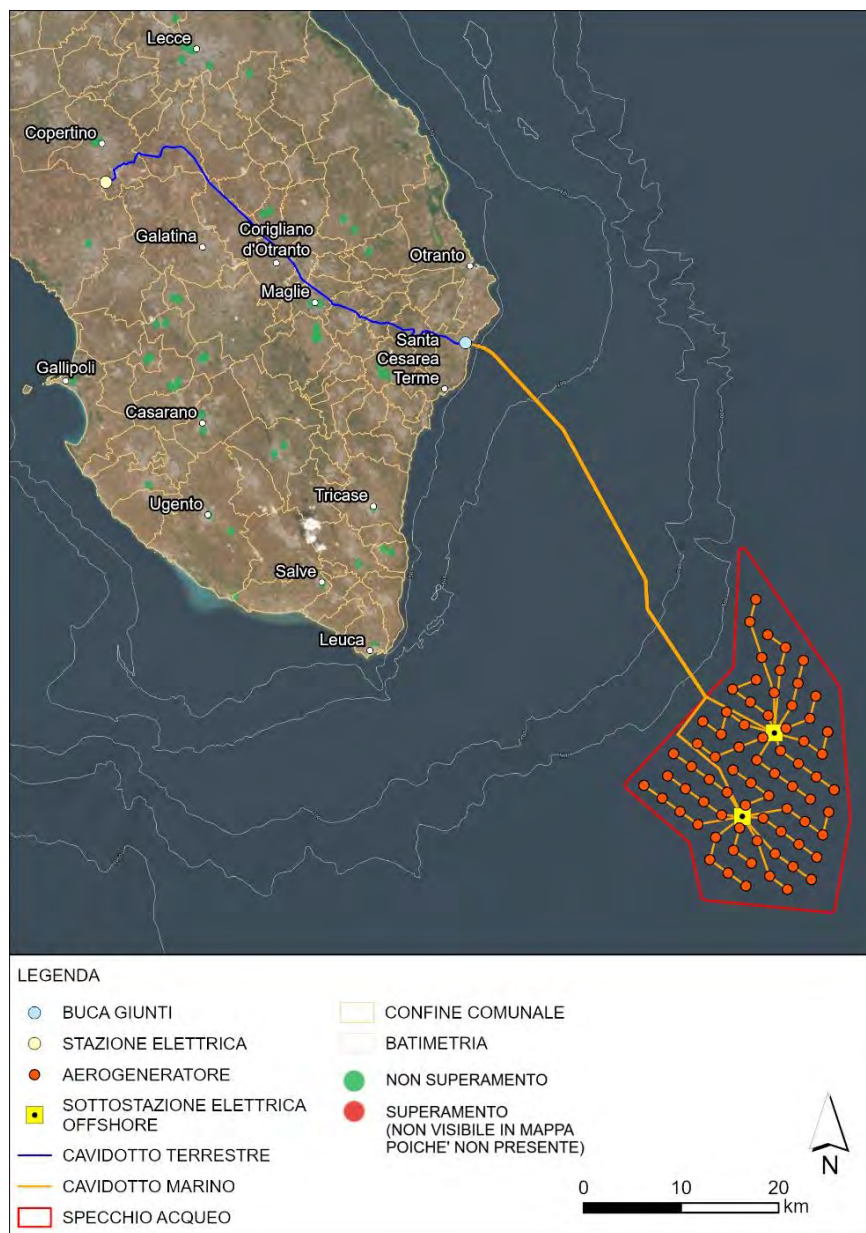
Figure 5-69 Map of electromagnetic field monitoring conducted by ARPA Puglia in the Area Vasta
